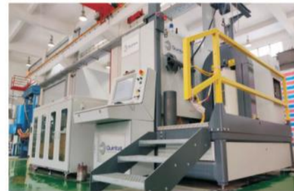
Hot isostatic pressing equipment
